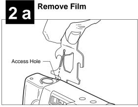
• Insert the punch end of the opening tool into the Access Hole.
